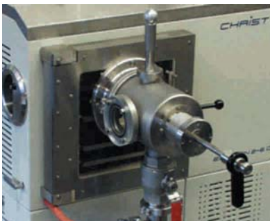
manipulator for retrieving individual vials during freeze-drying process (sample thief)
